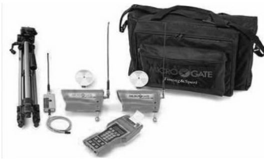
Fig. 5 – Handheld Microgate Timing System used at UMF Tîrgu Mureş with three passing gates.
